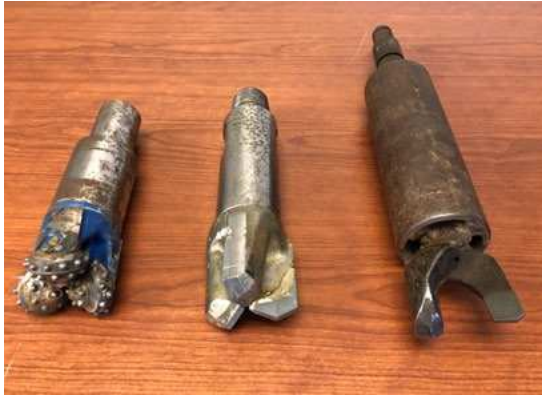
Figure 2. Cutting tools generally used: Tri-cone Roller Bit and Drag Bit. An example of a modified tool is: Two-wing Drag Bit with a guide tube
